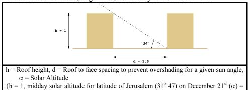
**Figure (12):** The Urban Canyon Sections - Urban Canyon Ratio (H/W): 1: 1.5.
