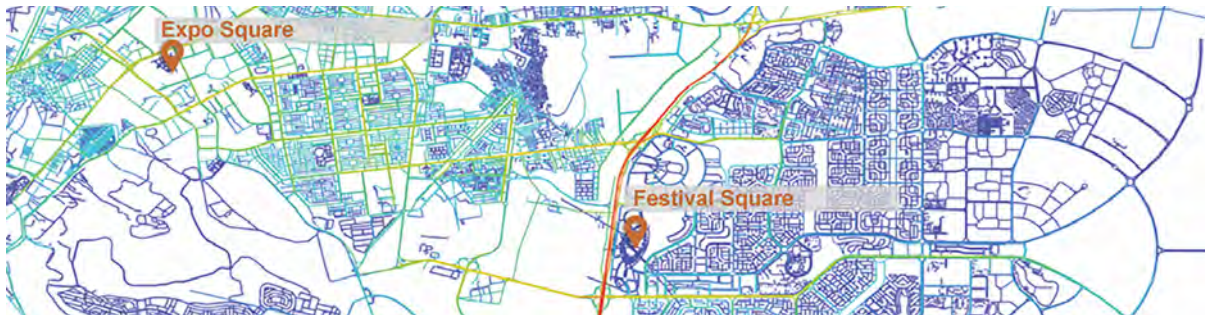
Fig. 6.45: The two Squares in relation to Spatial integration map (R7) of the connectors' network
