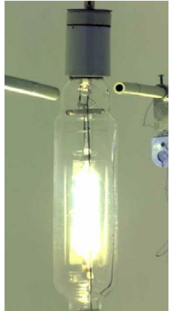
1,000W Metal Halide lamp in photometric test at Futek
