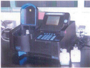
Plate 1. UV Spectro Photometer for sulphide, nitrogen and ammonia & phenol analyses.
