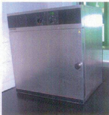
Plate 7. Oven , for oil & grease determination
