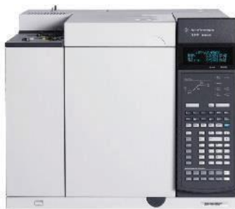
Fig. 5.5: Refinery and other petroleum gases containing H 2 , O 2 , N 2 , CO, H 2 S, CO 2 measurements
