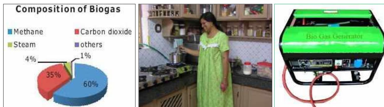
Fig (229): (left) General composition of biogas (middle) Housewife using biogas in cooking in India (right) Typical electrical generator based on biogas feeding –
