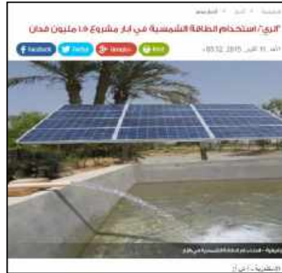
Fig(318): Using solar pumps for groundwater extraction in Million Feddan Project www.akhbarmasr.com
