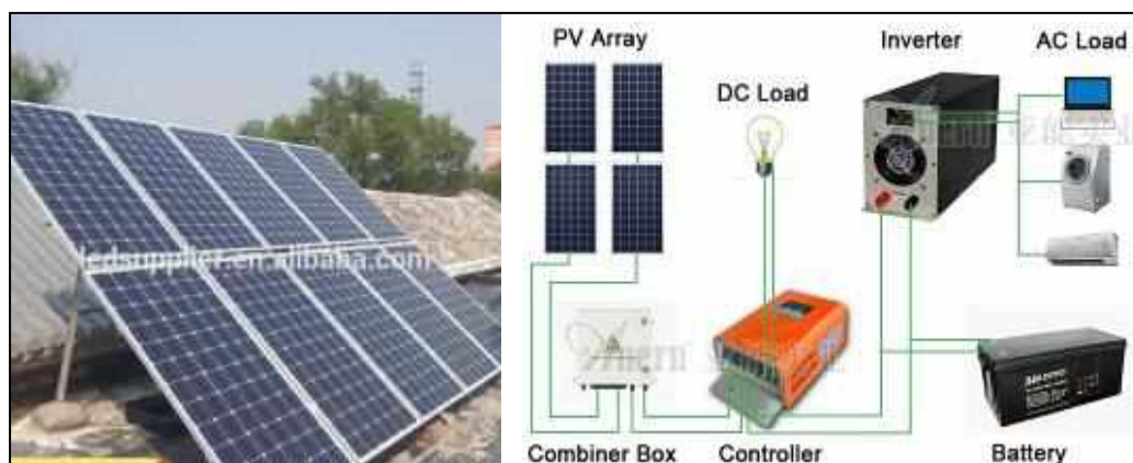
Fig(213): Photovoltaic System main components – Source: http://www.alibaba.com - retrieved 13/12/2015
