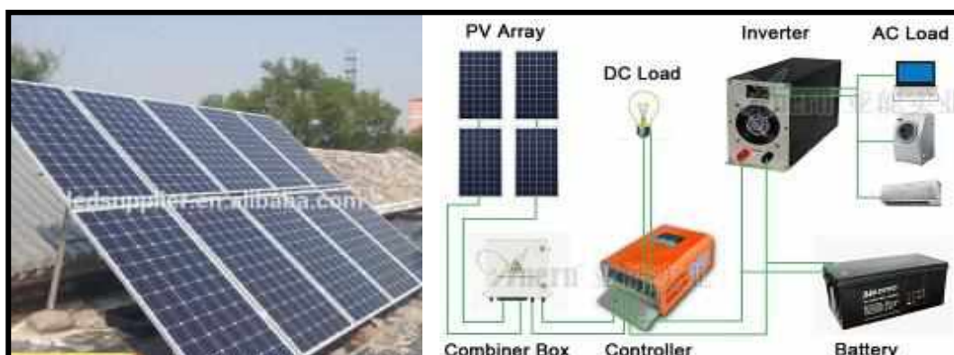
Fig(327): Solar PV System with all its components (as shown in the site of the manufacturing company). Source: Ref. No.10
