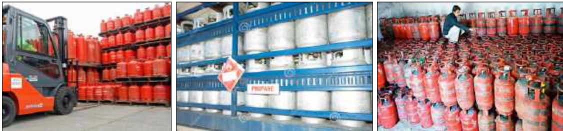
Fig (119): LPG cylinders vertical storage and caging practiced in South Africa, Us, and India
