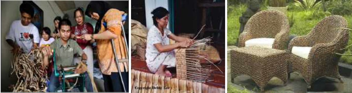
Fig(193): The reuse of wetland plants: processing dried water hyacinth stems for use as a material to make furniture in Sulawesi, Indonesia
