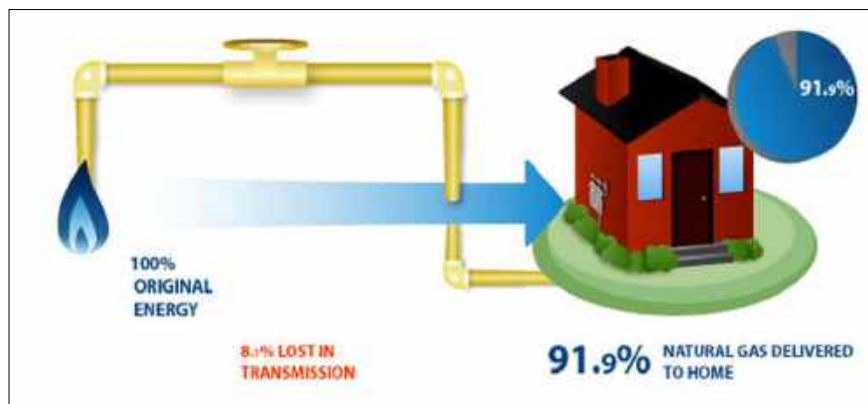
Fig (126): Household NG transmission efficiency as set by the American Gas Association (AGA)
