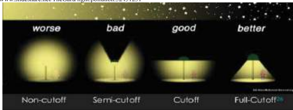
Figure A-8: Types of external luminaries light pollution
