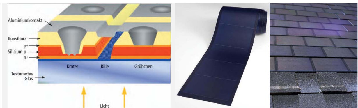
Fig. 1-41 Structure of Amorphous Silicon Cells // Forms of Amorphous Rolls // Rolls on roof (BIPV)
