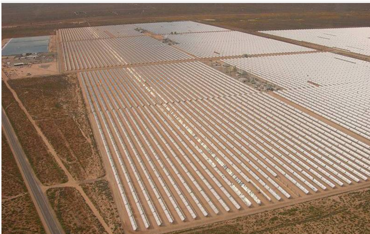
Fig. 2-3 The Large-Scale Concentrated Solar Collectors Plants With Electrical Generators, The Plant has Similar View With The Photovoltaics Plants, in California Desert, USA.
