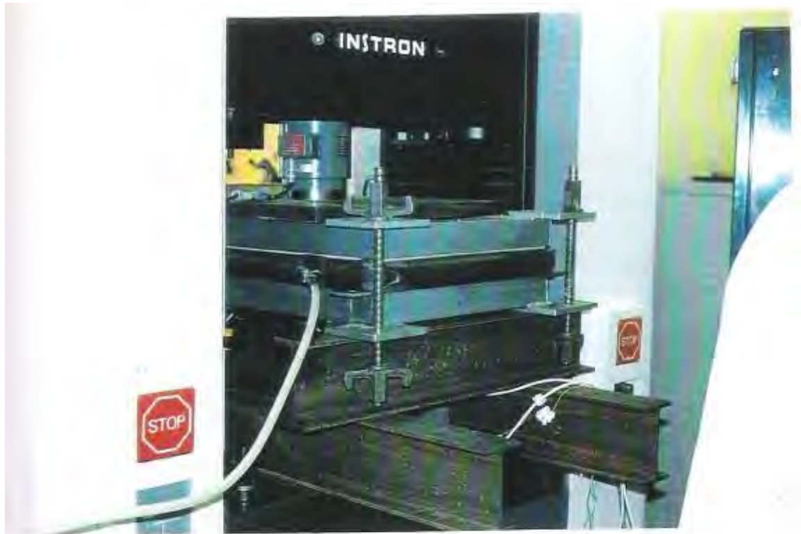
Figure 8.8 A photograph for the loading system showing air bag sandwiched between two frames .
