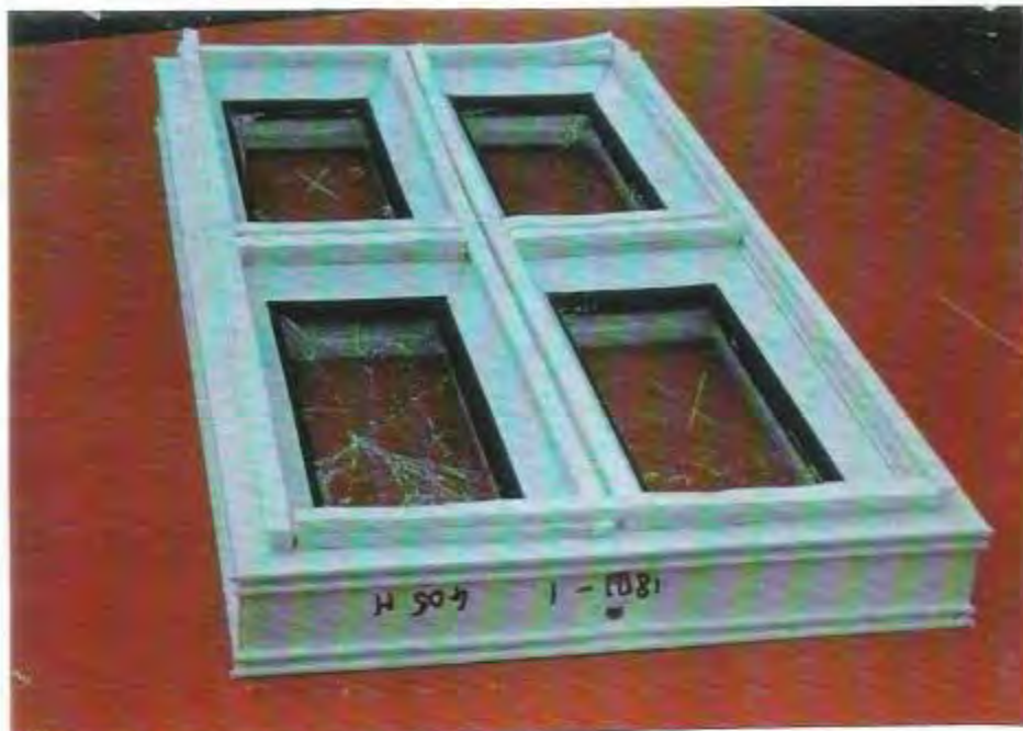
Figure 8.12.c the patterns of fractured glazing samples as revealed from the experimental test.
