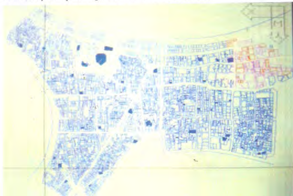
Fig.4-7, The surveyed map was digitised in an Autocad environment
