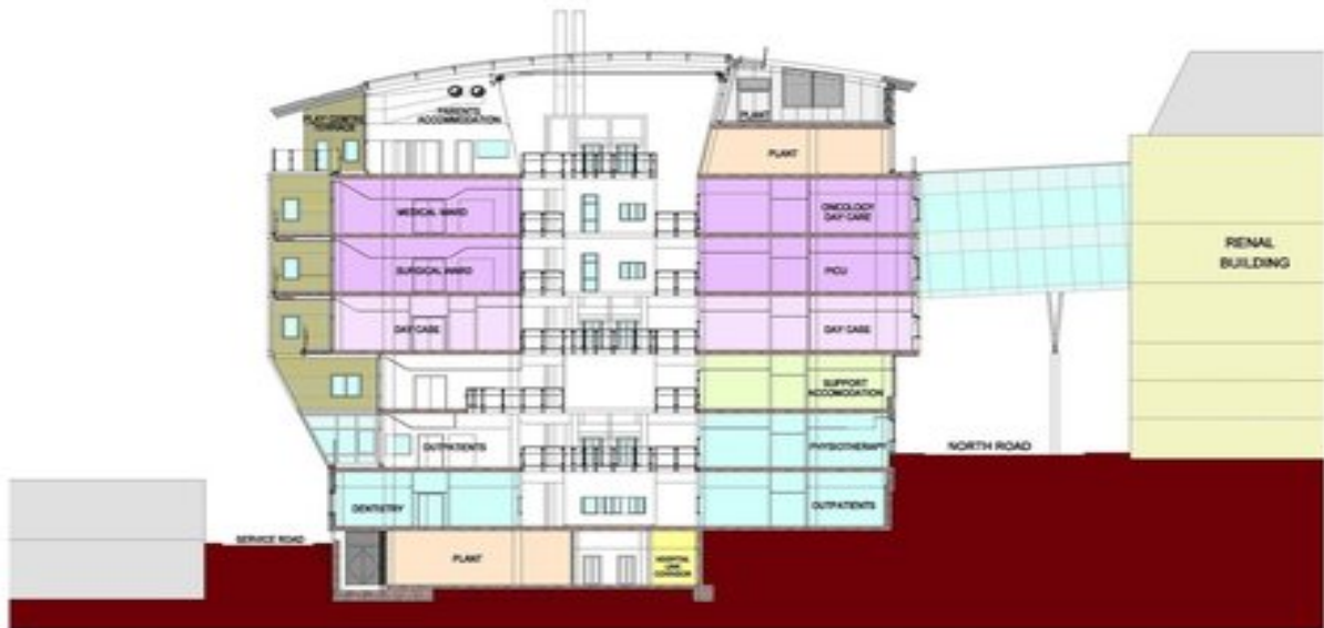
Cross Section Looking West
