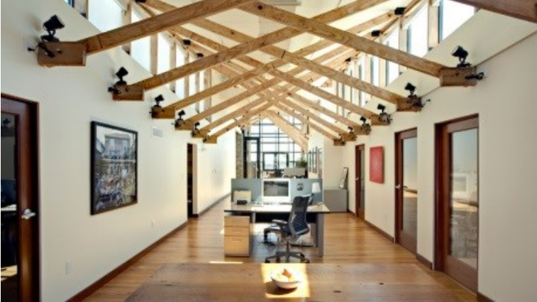
Figure 2-4 Clearstory light in plan and section source (arch daily adapted by researcher) planes (Figure 2-4) as it provided deeper penetration of light into the space. Clearstory light is a perfect light for gym halls, libraries, museums, and circulation spaces.
