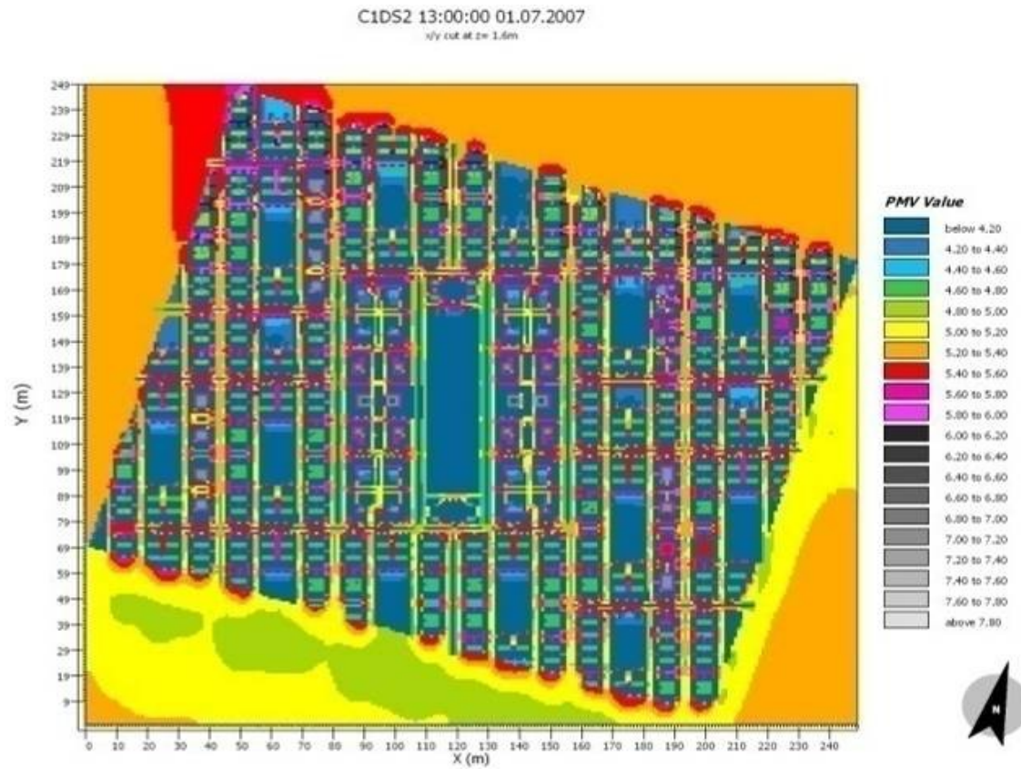
Figure (5-6/f): PMV mapping of C1DS2 1.6m a. g. l.at 13.00 LST.
