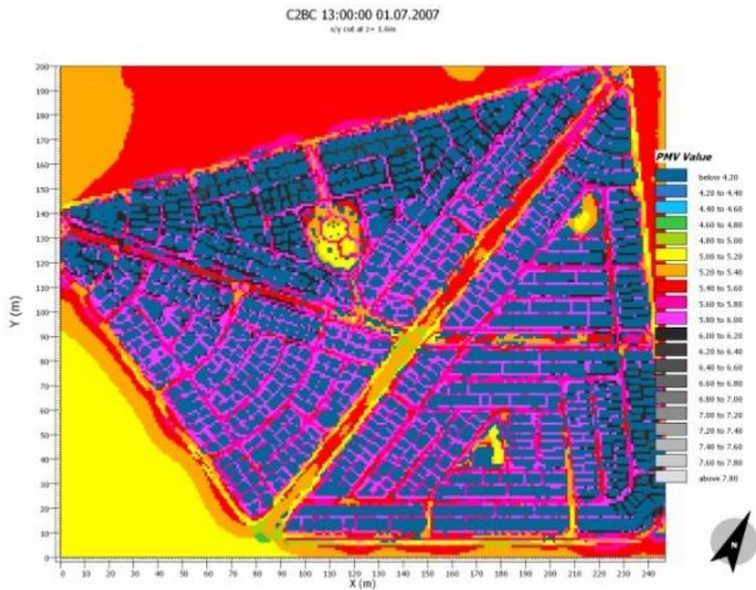
Figure (5-8/d): PMV mapping of BC1 1.6m a. g. l. at 13.00 LST.
