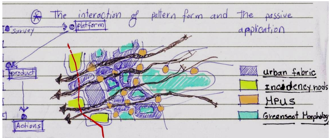
Figure vi: Freehand sketch of the author illustrating initial urban spatial design, i.e. usage of the urban passive tools into urban form to be capable of ventilation initiation due to pressure difference with orientation and aspect ratios, shadowing, evaporation and other passive cooling applications; the red axe line demonstrates that an urban form unit can be generated to produce pressure difference areas capturing amount of solar radiation, his has been published in (Fahmy and Sharples 2009a).
