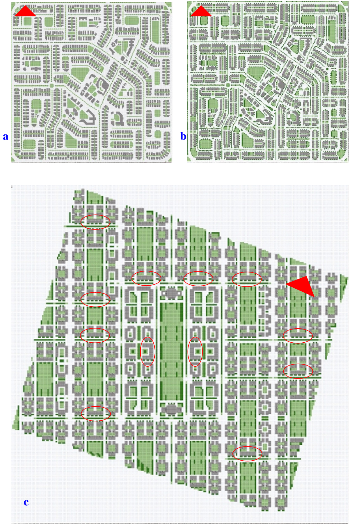
Figure (5-4/a, b, c): Master plans of BC1, C1DS1, C1DS2 and C1DS3 from upper right, left and down respectively; buildings in grey, grass in light green and trees in dark green. The red ellipses indicate the location of the high buildings used to help ISL-UCL mixing along with generating canyons' vortices.
