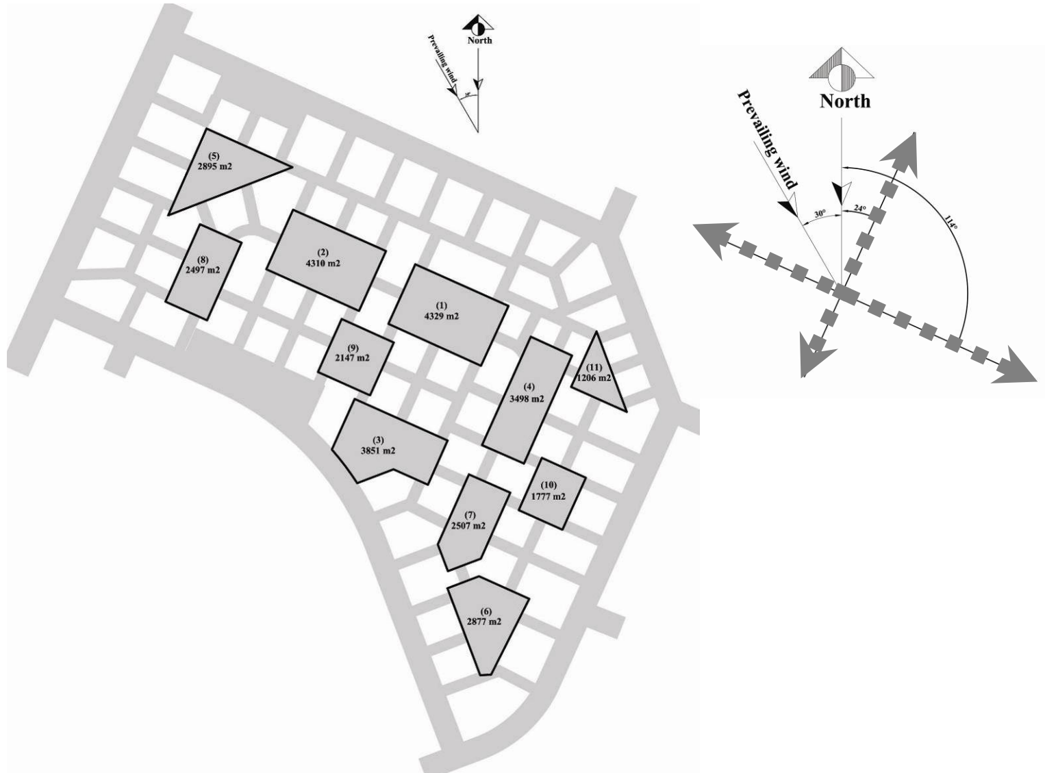
Figure 4-10: The case study master plan with the wind orientation of the majority of street illustrated
