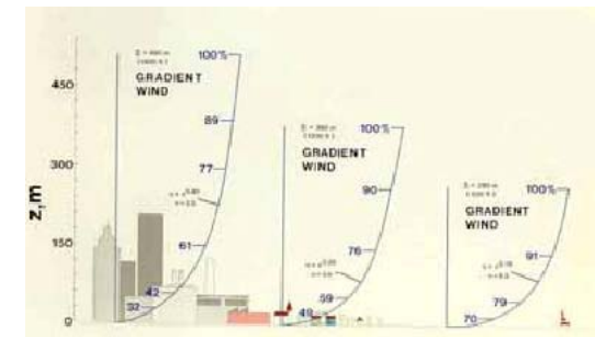
Figure 2-2: Diagrammatic wind speed profiles above urban, rural, and sea surface, after University of California [49]
