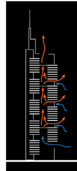
Figure 3-39: Sectional diagram of Commerzbank by Norman Foster illustrating the axi-symmetric venture approach, after Etheridge and Ford [145]
