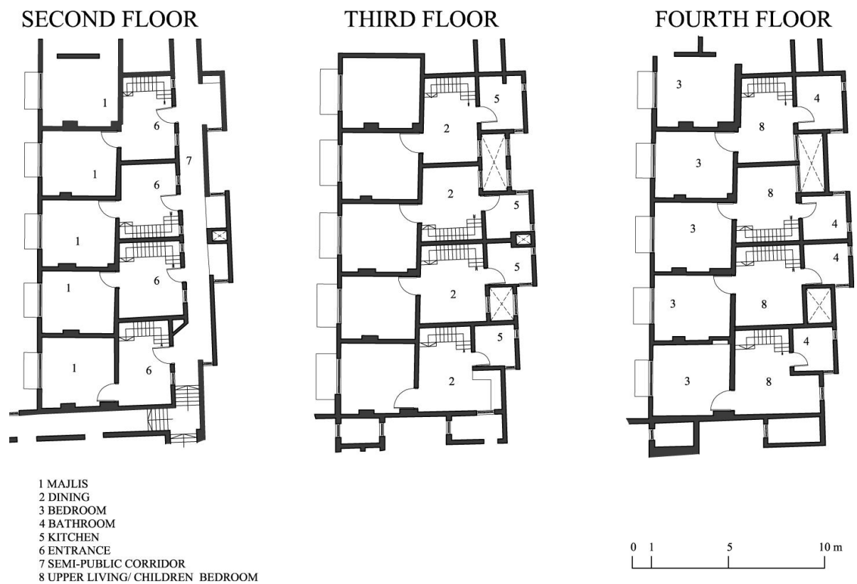
Figure 3.30 Plan of the Southern wing of the residential units in Wikālat Bāzar'ah.
