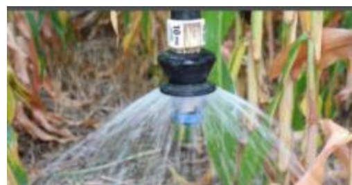
Fig. 5 – Rotating, Low pressure sprinklers
