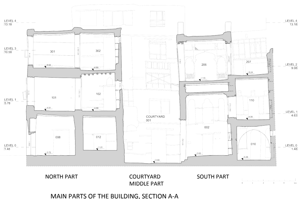
Fig. 21 Section through the building. Notice the double floor system between the iwan and room 206, and the whole South part leaning into the courtyard.
