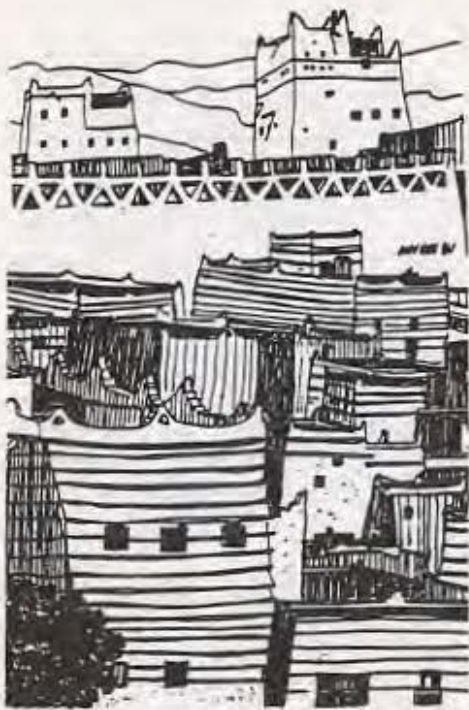
Fig. 19 Sculpturesque Mud Parapets in Aziv, Saudi Arabia. On roof tops and terraces the railings and parapets are often moulded to create sculpturesque forms. Edges of the parapets are rounded and finishing points of roofs and terraces are decoratively moulded.
