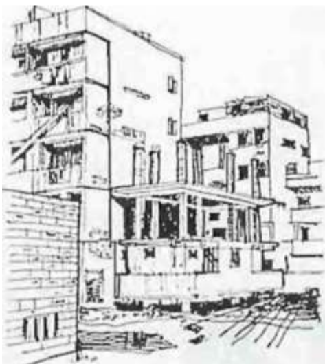
Cairo-Helwan u The informal actions are actuaJJy the iohabitanrs procedure in soll'ing the existing problems by 'Self help . The abon figure shows the extension of an exist ing dwelling by the erection of a new building adjacent to the exi. tin one.
