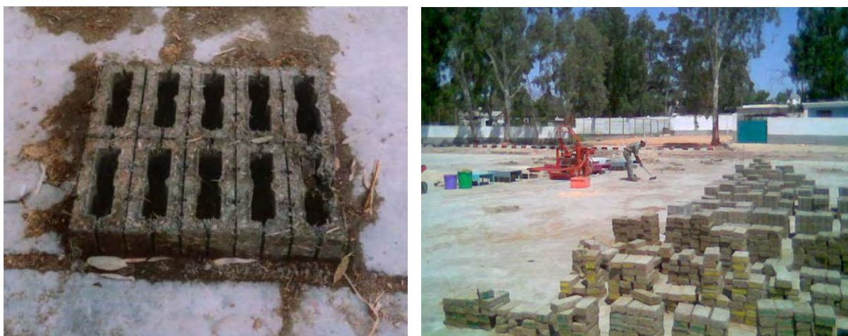
Fig. 2: Unsuccessful hollow and successful solid rice-straw based brick.
