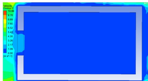
Fig. 11 A contour section shows that no air movement inside room.
