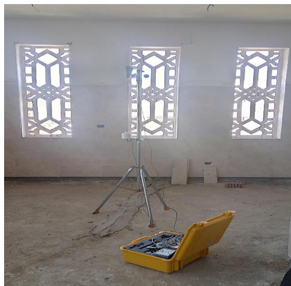
Fig. 9 indoor measurement by Nova-Lynx weather station
