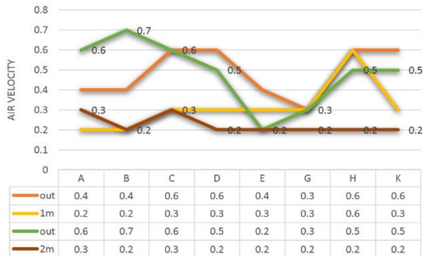
Fig. 27 A diagram of air velocity at points from A: K due to natural ventilation at positions 1 and 2.
