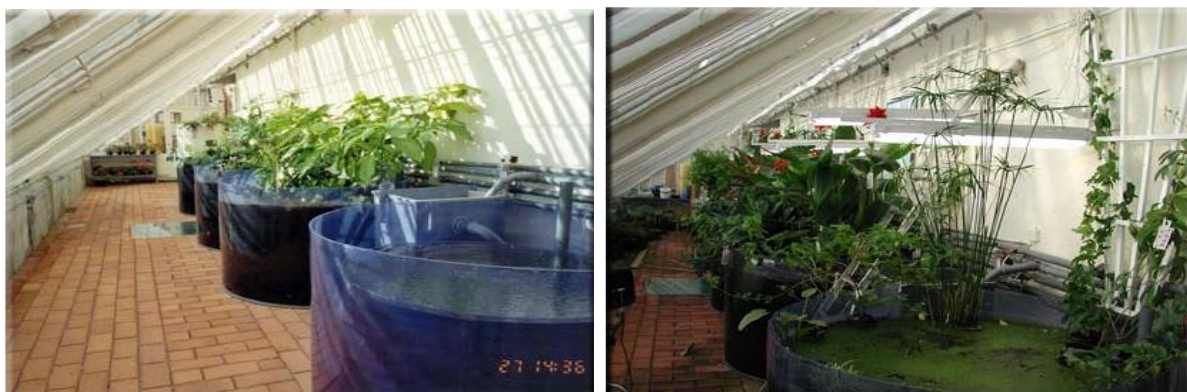
Fig.19: Hydroponics used in central wastewater treatment plant in Sweden-Treatment of domestic wastewater using microbiological processes and hydroponics in Sweden-Anna Norström-Stockholm 2005
