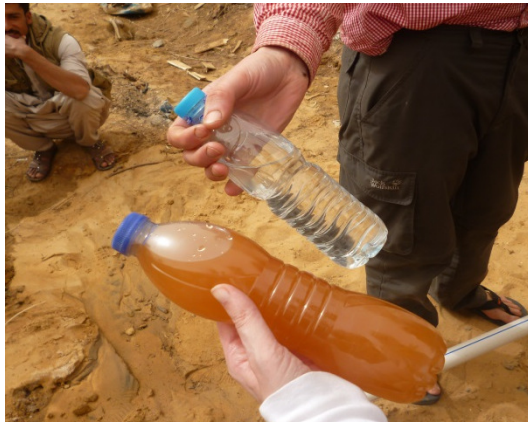
Figure 3: Iron sludge removed from filter and clear drinking water in Egypt.
