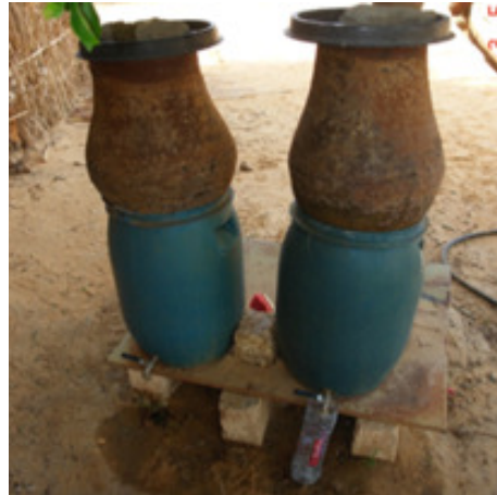
Figure 3: Example of local residents’ use of clay pots filtering water that is then caught in plastic buckets.
