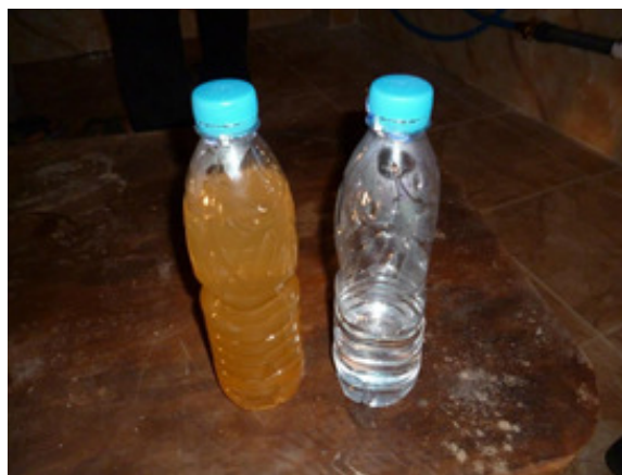
Figure 1: Backwash water displaying the high iron content (left) and water after filtration. Both samples are from the oasis of El Heiz in the Western Desert.
