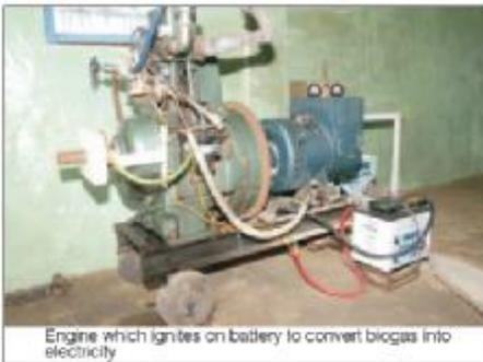
Engine which ignites on battery to convert biogas into electricity
