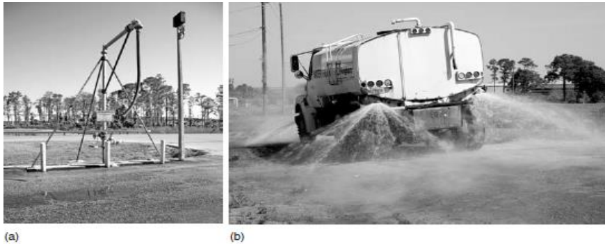
Figure 73 Treated water use for street cleaning and dust control: (a) treated water filling station for street cleaning vehicle and (b) water truck spraying treated water (Asano, Burton, Leverenz, Tsuchihashi, & Tchobanoglous, 2007)
