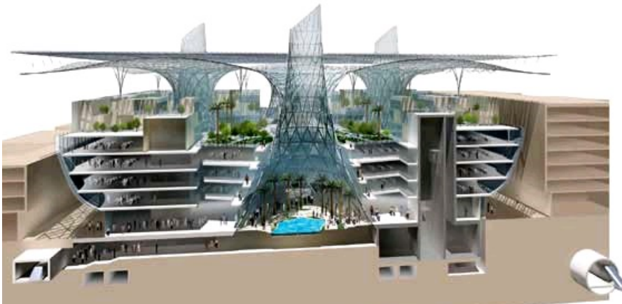
Figure 5- A rendering shows a cross section of the Masdar Headquarters, A series of bellshaped wind towers ventilates the building 83
