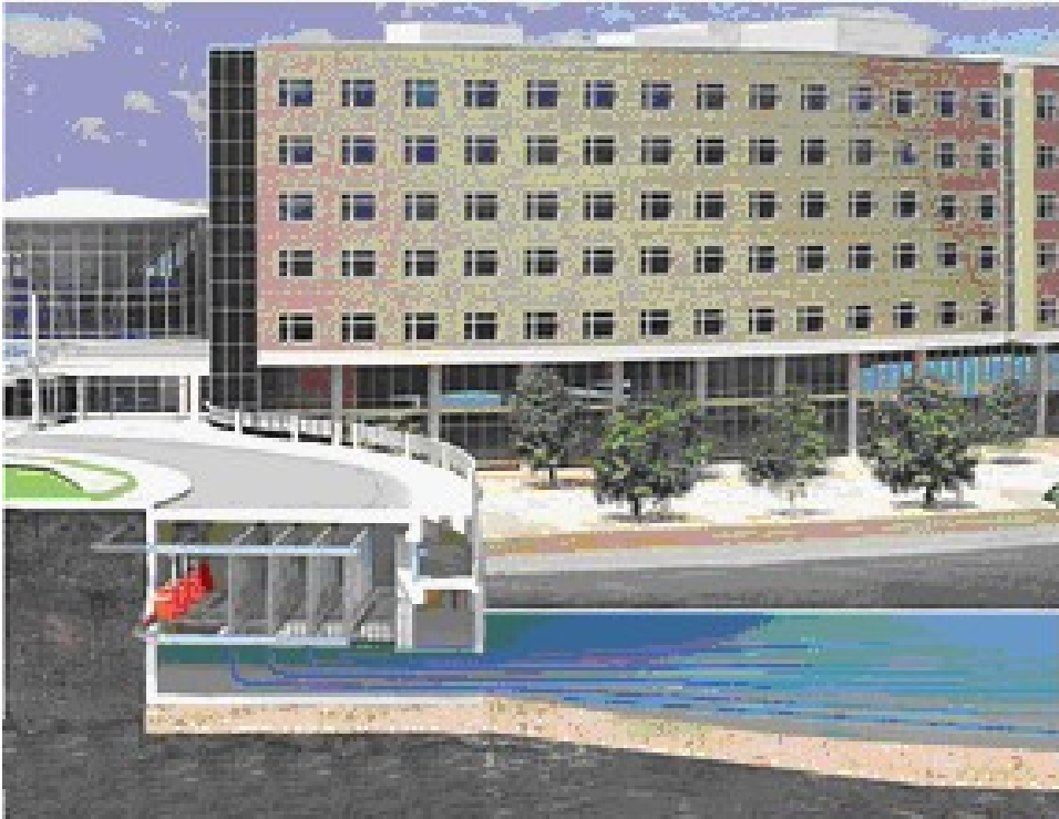
Figure 2- section in the geothermal heat exchange tubes, application, Sherman hospital, Elgin, Illinois, 2009 57
