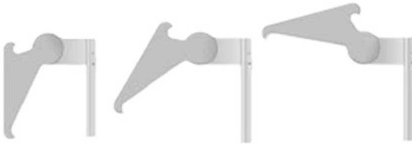
Figure 4- Automatically controlled metal louvers rotation with sun angels 0-90 degree 21
