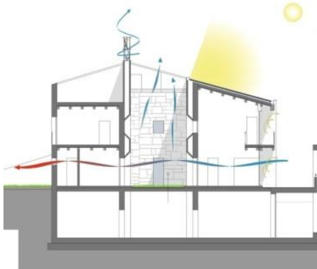
Figure 1.13- Providing cross ventilation through courtyard 3
