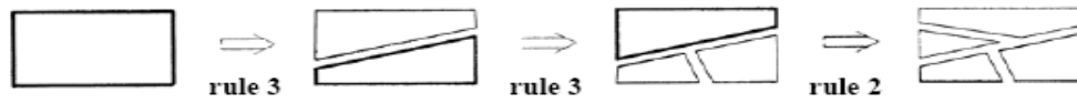
Fig. 2.9: A derivation using the third and fourth rule of ice-ray grammar. Source: Stiny, 1977.
