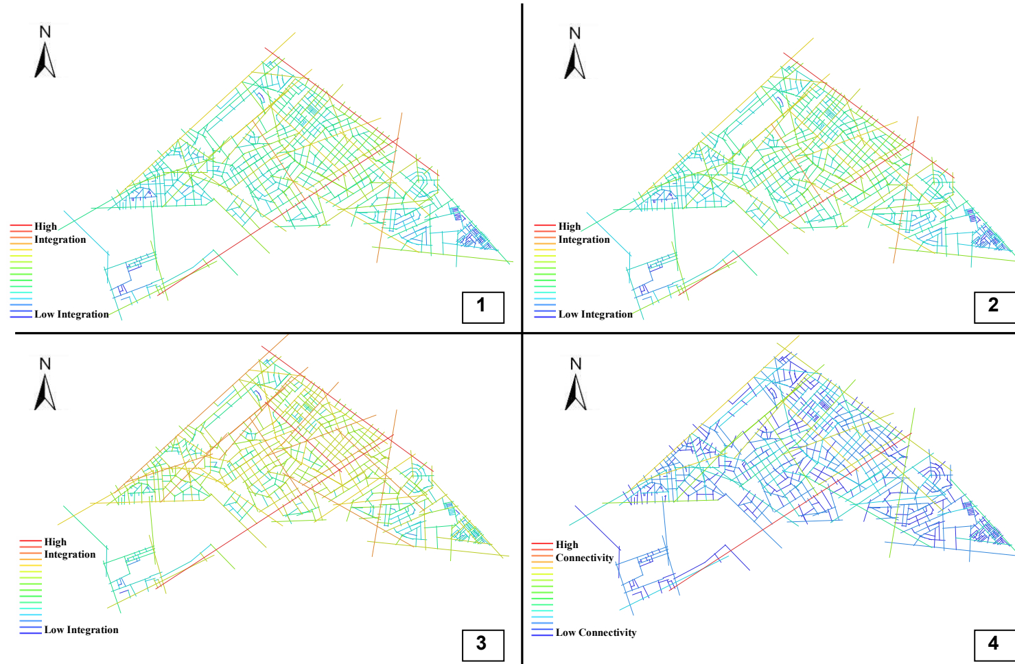
Figure (4-10) Spatial analysis of Misr el Gadida district 1- Global integration ( R=n ) 2- Local integration ( r=10 ) 3- Local integration ( r=3 ) 4-Connectivity
