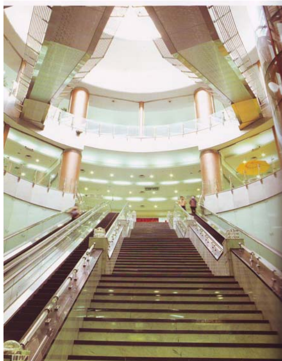
Fig (2.25) Dome interior at Noksapyeong station, maximizing influx of light and its effect, after light is influxed into four underground stories through the dome, it reflects from glass finish. [10]
