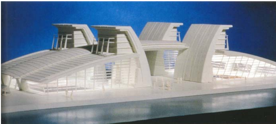
Fig (3.28), Kowloon Station, Concourse roof model. The roof is anchored by four towers that create a monumental open space between them, a gateway to the stations. Light is taken to the catacombs of the platforms via diagonal paths of deflected light.
