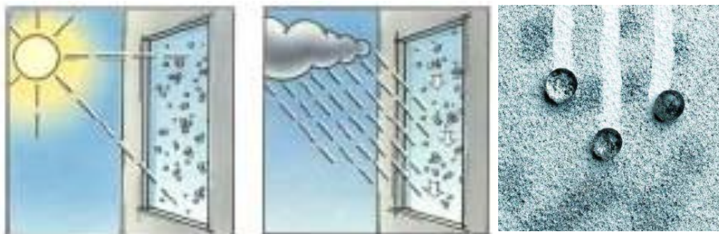
Figure 3.40 Left, organic dirt and grime is broken down by exposure to sunlight and left clean surface. Right; self-cleaning effect on surface.
