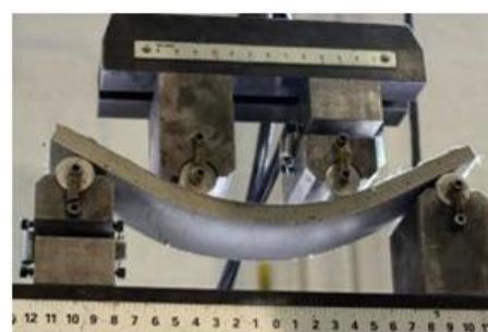
Figure 3.30 Concrete under force, small and narrow cracks happen instead of one big crack.
