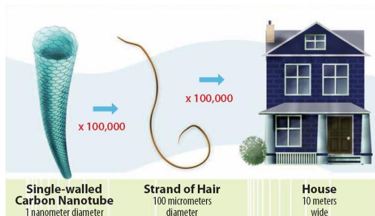
Figure 3.18 The diameter of carbon nanotubes is to the diameter of a hair as the hair's diameter is to house wide.
