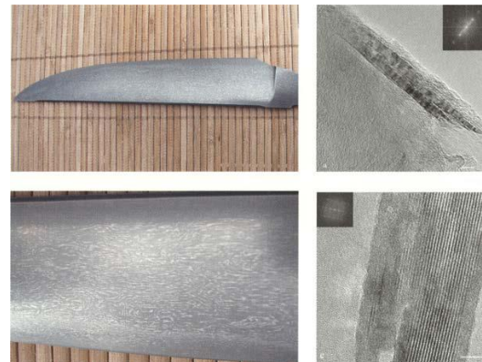
Figure 3.26 From macro to nano. The four images of parts of a Damascene sabre show that the blade is made of -carbon nanotubes which responsible for the extraordinary strength and flexibility of the steel.
