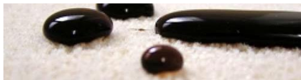
Figure 3.53 Carpet produced by Nanolia Textile, with waterproof properties.
