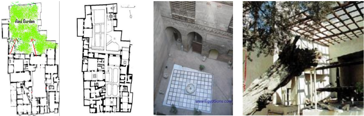
Figure 23: The gradual form of the mass creates more top surfaces which were used as roof gardens. Bayt Al-Soheimy, Cairo, Egypt [45, 46]
