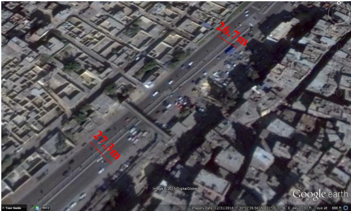
Fig. ( 210): Shows a shot taken by Google Earth for the Nasr rd. in front of Manshiet Naser and the cemeteries and their the width of the road has been measured to find out that it is of 26-27m.
