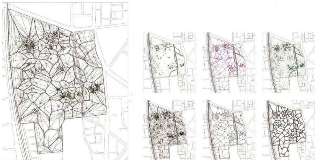
Figure 3.9 Right: the main layout. Left: the stages of generating the layout starting from the points to the final form.
