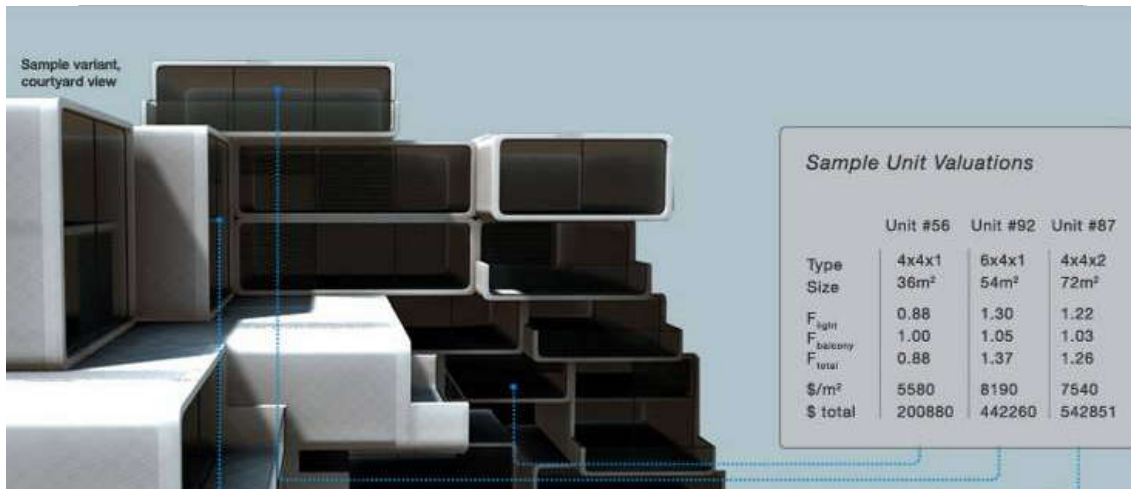
Fig. 4.46 The construction rule parameters are altered recursively with the goal of increasing the building value.
