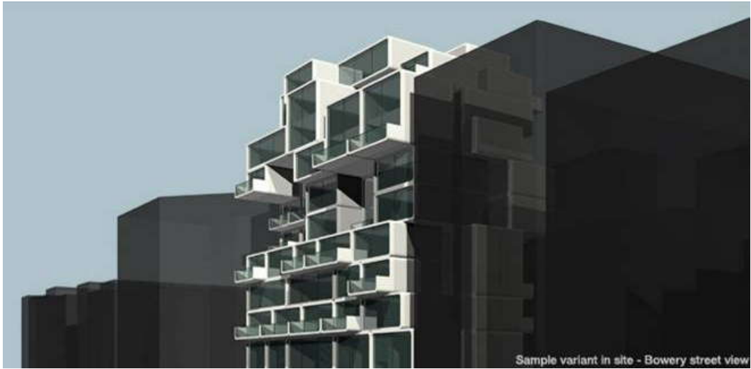
Fig. 4.44: A building variant is assembled out of pre-defined apartment types based on a series of construction rules.
