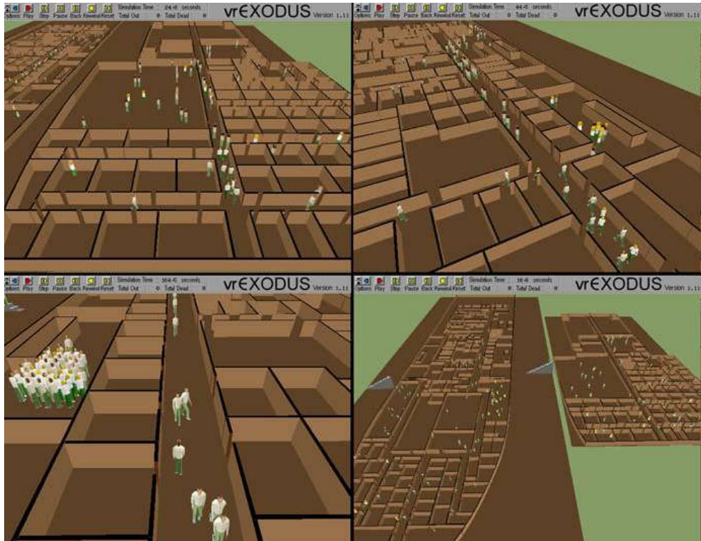
Fig 3.49 Simulation of a ship evacuation, using the tool EXODUS based on swarm intelligence.
