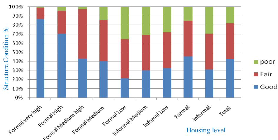
Figure 6-2: Distribution of buildings by structure condition by housing level
