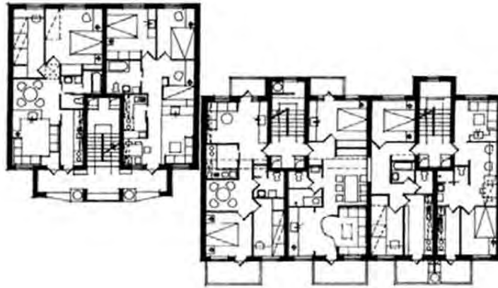
Figure 67 : Building with various dwelling layouts, drawing of M & A Architects, 1994, Pipe-Stairwell Adaptable Housing ,Cuiwei Residential Quarter, Beijing, China – Ref: Stephen Kendall, Residential Open building
