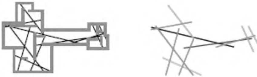
Figure 124: Linear representations (axial maps) of a settlement and a building plan. Note: More integrated lines are shown in darker shades.
