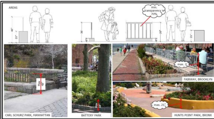
Figure (6-20) Bollard and railing. Source (www. nyc.gov/)
