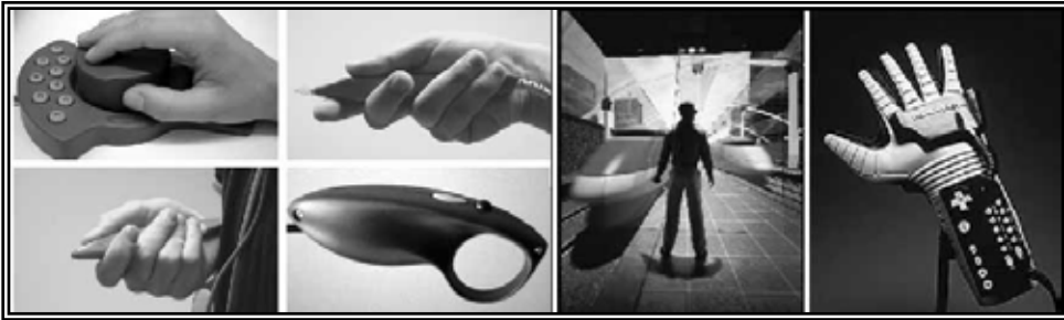
Figure (7-16) Interaction devices: Spacemouse, Stylus, holobench set-up, Stylus, HMD set-up, Hornet and data glove. Source (Honjo T., et al., 2006)
