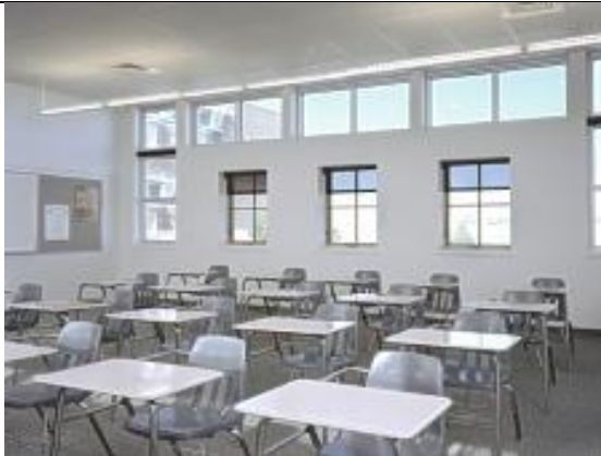
Figure 4. 56 Most of the lighting for classrooms is natural, and operable windows allow fresh air inside without disrupting the heating, ventilating, and air conditioning (HVAC). "Sustainable School Book". 3
