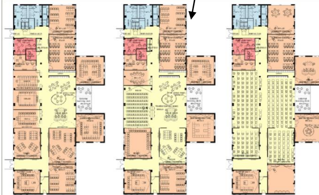
Figure 3.34 Cluster floor plans The drawing shows the variety of different layouts the plan can support for different curriculum arrangements. The same furniture is used in each of the layouts, presentation and exam scenario. (Adaptability). “www.cabe.org.uk”
