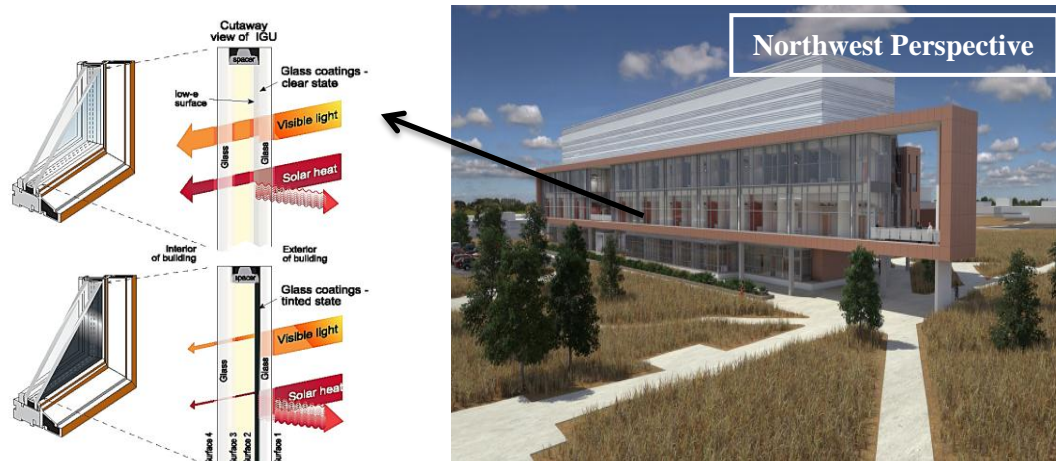
Figure 4.7 High Performance Glazing in Argonne National Laboratory (North and West Façade) Source: Argonne National Laboratory, URL: http://web.anl.gov/esb/index.html , accessed April 5, 2013.
