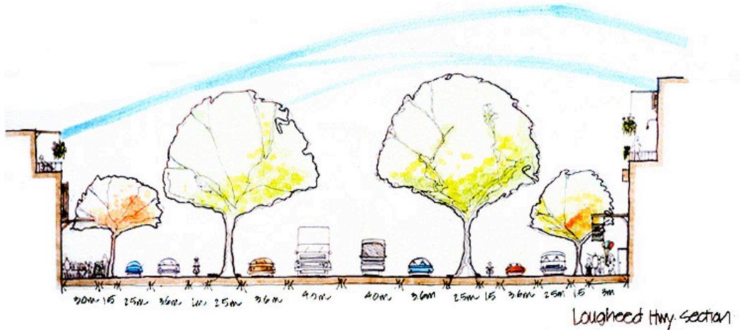
fig(5-21): This section shows how the existing right-of-way is utilized so that the amount of roadway given to cars is greatly reduced. Cars, trucks, and buses are given a 14.4 meter paved roadway, which accommodates four lanes of two-way traffic. Landscaped boulevards on either side separate the high-traffic zone from the slow-speed, pedestrian friendly parking lanes.
