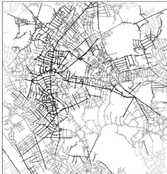
Figure3. 8. Example of axial map analysis according to space syntax technique: Darker lines is the most integrated, while light gray is segregated (source: Kim Y O, 1999 ).
