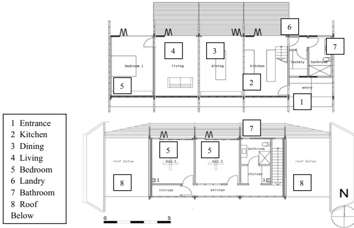
Figure (4.12) Lara Calder eco house plans (ground, and first floor) scale 1/200 (Lara Calder, 2008)
