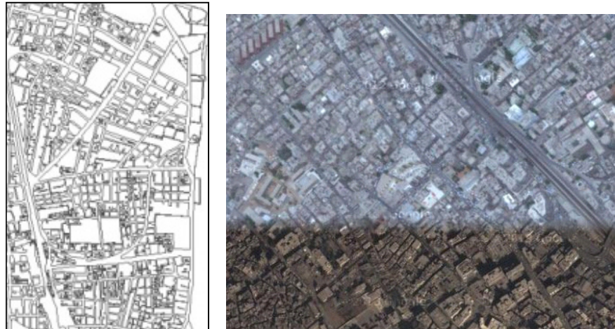
Figure 6.69: Applying the grid and circular system of planning streets and the absence of hierarchical planning system in the middle area support the visual and physical permeability
