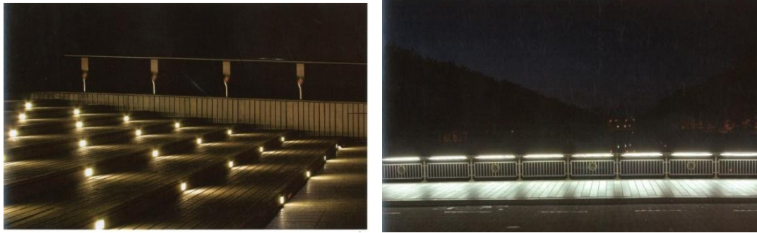
Figure 5.52: Left: the use of dark floors. Right: The use of bright floors is more appropriate for lightening the steps and pavements.
