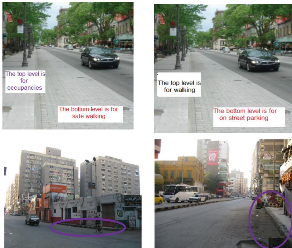
Figure 6.90: Left: The use of two levels pavement in the retail and mixed use streetscape. Right: The use of two levels pavement in the residential streets. All pavements should have safe access points that are suitable for all kinds of users
