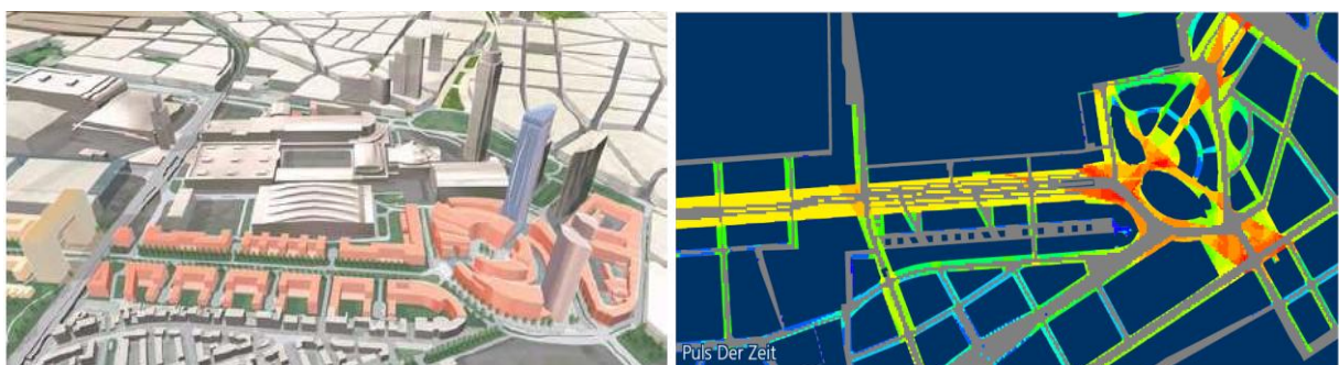
Figure 5.12: Left: Computer model for a new boulevard in the central Frankfurt, Germany. Right: Fathom analysis of the visibility of pedestrian spaces in one of the four design options for the public space of the Boulevard ( www.intelligentspace.com )
