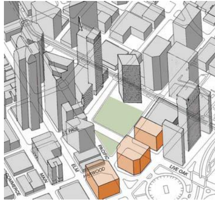
Figure 5.51: It is proposed to locate the towers and open spaces in different angles in order to impart dynamic light and shade across the site and to avoid blocking the views from the street level.
