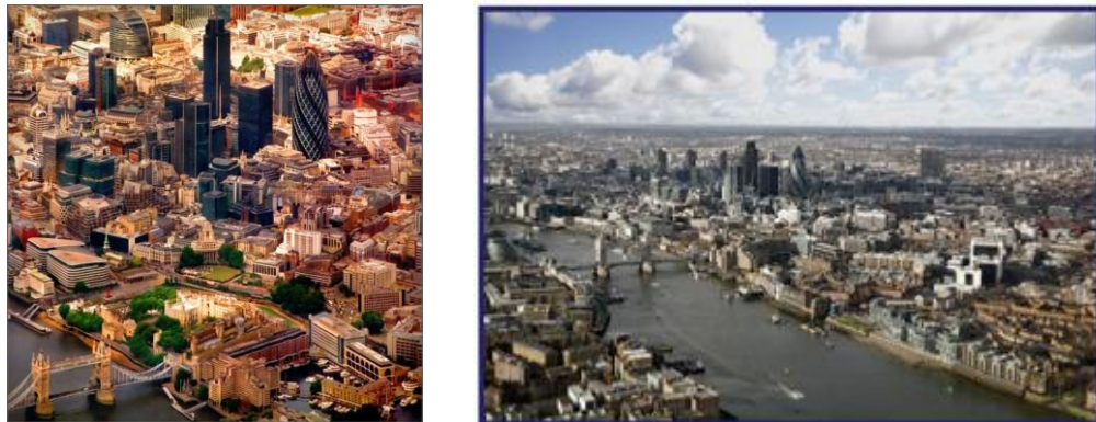
Figure 2.7: A comparison between low oblique and high oblique images. Left, low oblique image of London, UK ( http://www.flickr.com ). Right, high oblique image of London shows the horizon and sky line of the city ( http://www.aerolens.co.uk )
