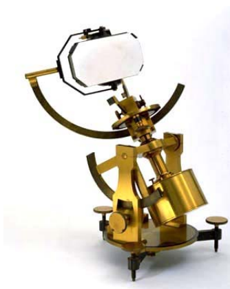
Fig (4-1): The optical system “Heliostat” designed by the Frenchman J.T. Silbermann in 1843.
