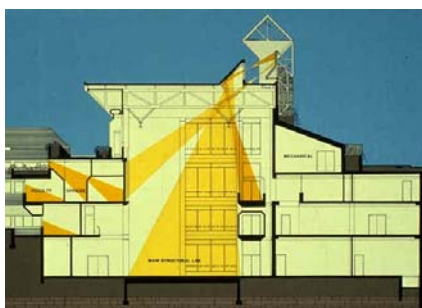
Above: Cross-section showing the illuminated zones Below: Sun angle 24°-47°
