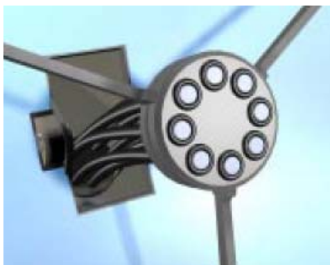
Fig (4-74): Close-up view of the large-core optical fibers end.
