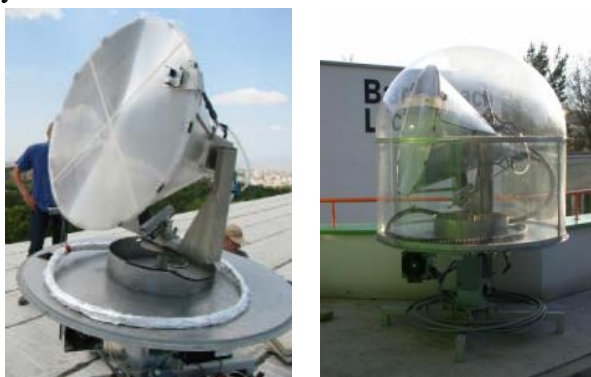
Fig (4-79): Solux Lighting System heliostat. (With and without the acrylic dome)
