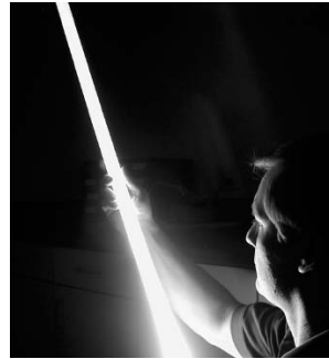
Fig (4-75): Cylindrical diffusing rod (designed and constructed rod)
