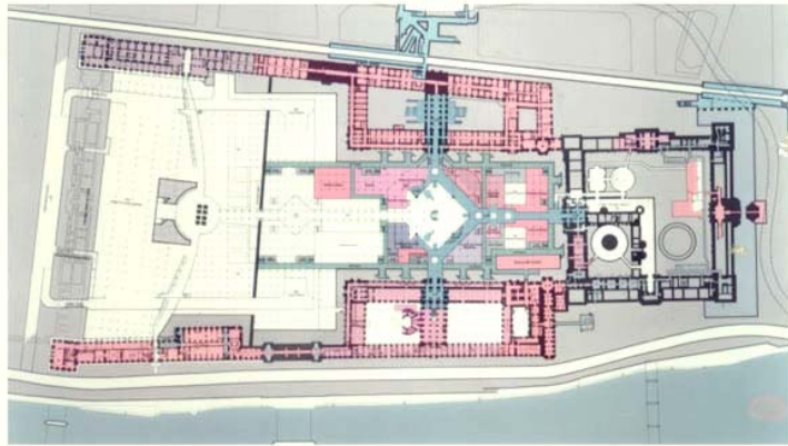
Fig (3-60): The Grand Louvre underground extension plan showing Phase (I) major components.
