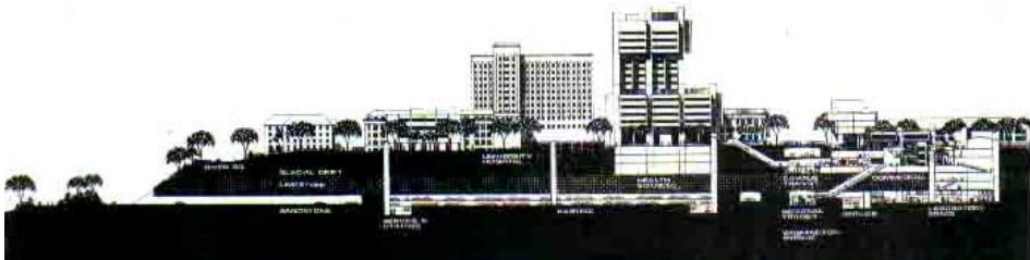
Fig (1-37): Concept for the underground development at the University of Minnesota. (Drawing John Carmody)
