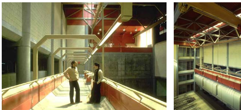
Fig (4-38): Walkway through the main structures lab illuminated by the passive solar system and supplemented by fluorescent luminaires.
