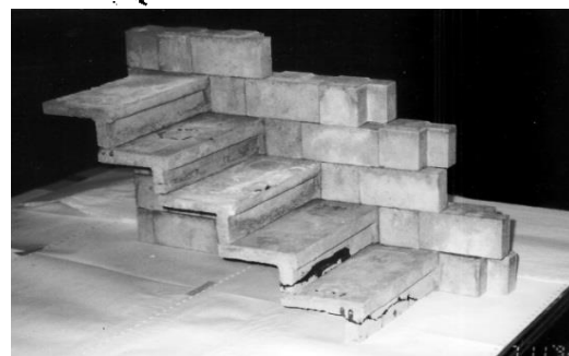
(Fig 11) Photo of .the step/block self build stair.
