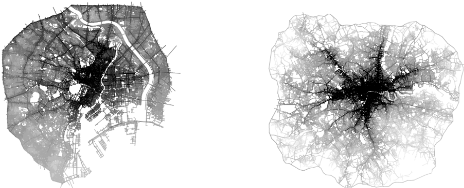
Figure 2.5. Cities of Tokyo (left) and London (right) have similar foreground networks of a ‘deformed wheel’ pattern while having two different background structures reflecting the spatial dimension of cultural differences(source: Hillier, 2009b).
