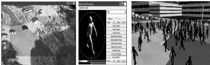
FIGURE 1. HUMAN MODELS CROSSING AN INTERSECTION: A SCREEN SHOT IMAGE OF A SIMULATION TOOL (LEFT), AN ANIMATED 3D CHARACTER MODEL (MIDDLE), AND A SCREEN SHOT IMAGE OF 100 PEOPLE CROSSING IN A VR MODEL.
