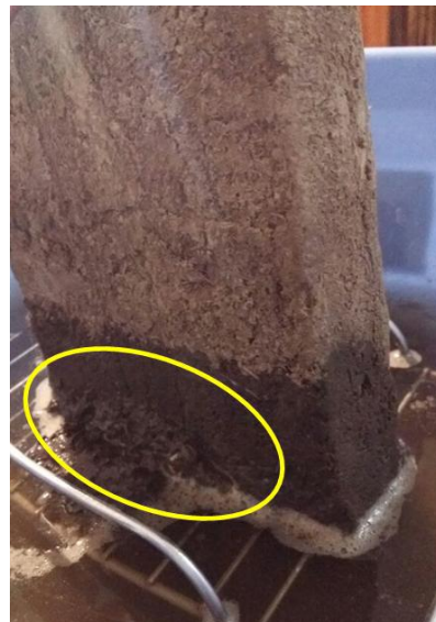
The first experiment of water absorption for Adobe bricks made of Palm leaves.
