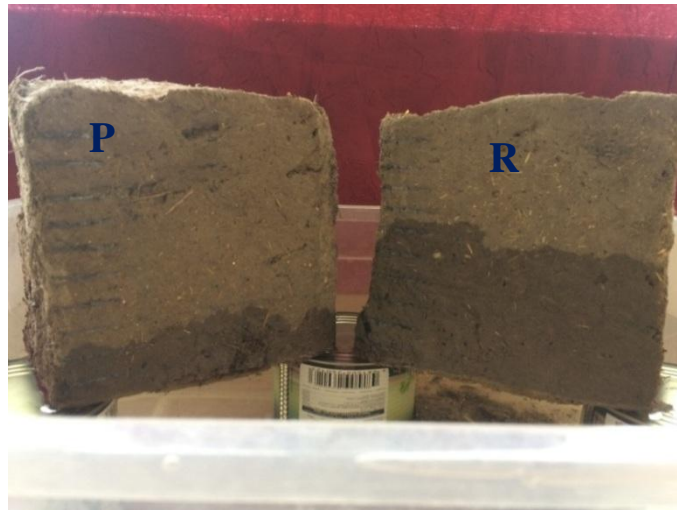
Figure 17: After an hour of the test, the Amount of water absorbed in both bricks. Author
