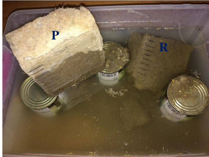
Figure 19: After 12 hours, the final result is the collapse of the rice straw Adobe brick, Author
