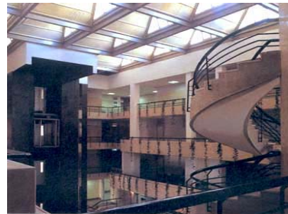
Fig (27): Atrium distributes daylight to building zones
