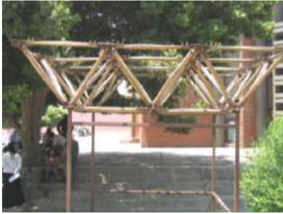
شكل 5- 41 نموذج الجمالون الفراغي بحر 3 متر المصدر: Raga, Tamer, 'USE OF PALM MIDRIBS AS STRUCTURAL ELEMENTS' (MSc Thesis, Ain Shams University, Department of Engineering, 2010), p. 60.
